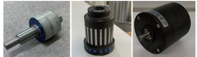
(a) Inner rotor (b) Pole piece rotor (c) Magnetic gear
