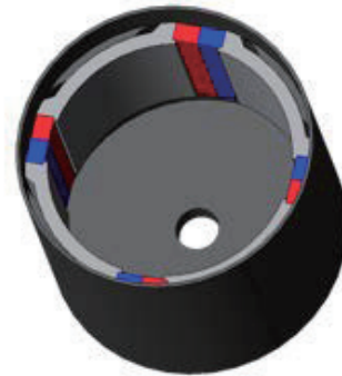
(a) Improved rotor of the segment PM motor
