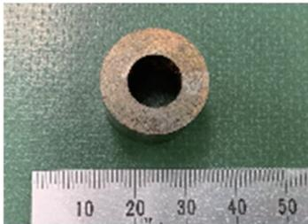
Fig.1 NANOMET® laminated ring core.
