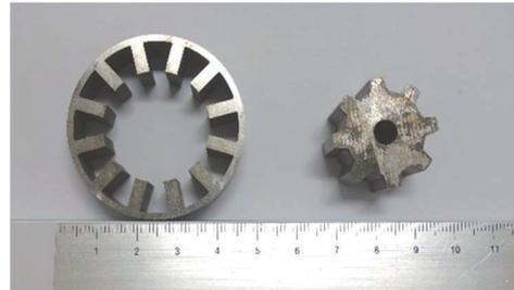
**Fig.9** Stator and rotor core of prototype 12/8 SR motor made of NANOMET® laminated alloy.
