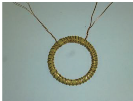
Fig. 1 Winding coil on ring sample without polymer case (photo).
