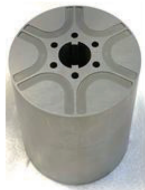
Fig. 5 IPMSM rotor with injection molded Sm-Fe-N bonded magnets ( \Phi 60 -L50).
