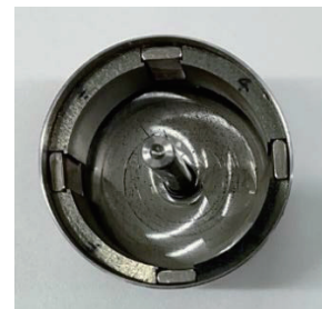
Fig. 8 Appearance of the rotor of the prototype segment PM motor.
