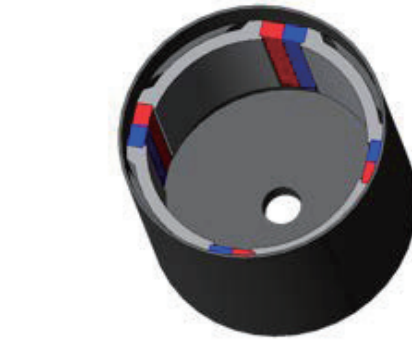
(a) Improved rotor of the segment PM motor
