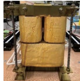
Fig. 5 Appearance of prototype orthogonal-core-type variable inductor consisting of cut core and laminated core.
