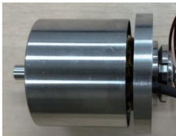
(a) Appearance of the prototype segment PM motor
