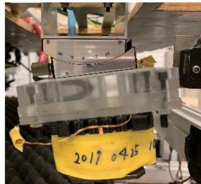
**Fig. 7** Tilted electromagnet for levitation control.
