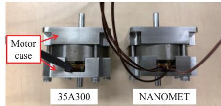
Fig. 8 Appearance of the prototype inset PM motors.
