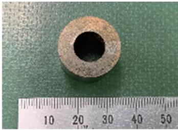
Fig.1 NANOMET<sup>®</sup> laminated ring core.
