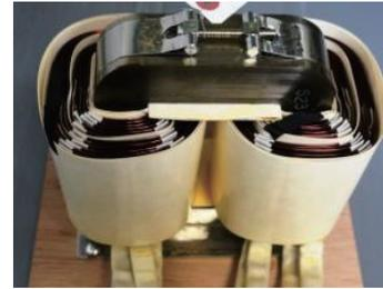
Fig. 4 Appearance of the transformer with non-interleaved winding.
