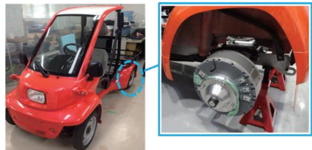
Fig. 1 Compact EV with in-wheel AFSRMs.
