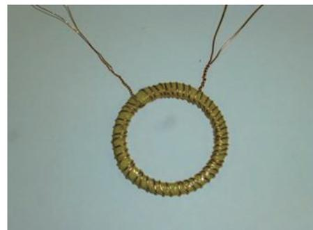
Fig. 1 Winding coil on ring sample without polymer case (photo).
