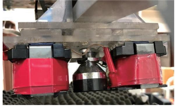
Fig. 3 Photograph of electromagnet.
