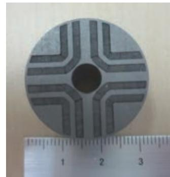
Fig. 7 Rotor core of the prototype IPM motor.
