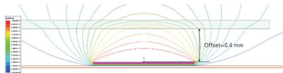
(b) magnetic flux line on 1.2 mm probe
