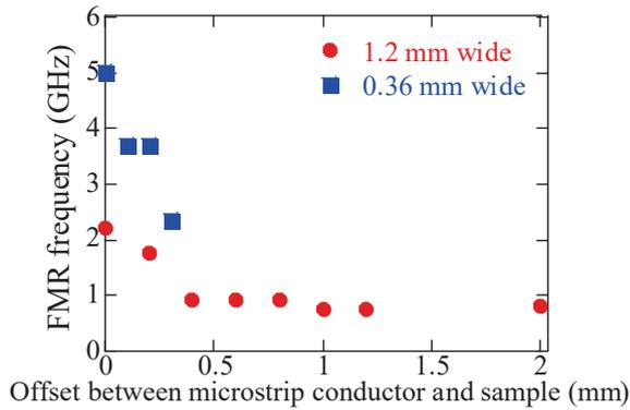
**Fig. 7** The FMR frequency as a function of the offset between the microstrip conductor and the sample (NiZn ferrite sheet).
