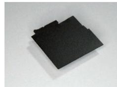
**Fig. 6** Photograph of NiZn ferrite film. This sheet is around 0.1 mm thick, and ferrite particles are contained in the polyethylene film<sup>23)</sup>.
