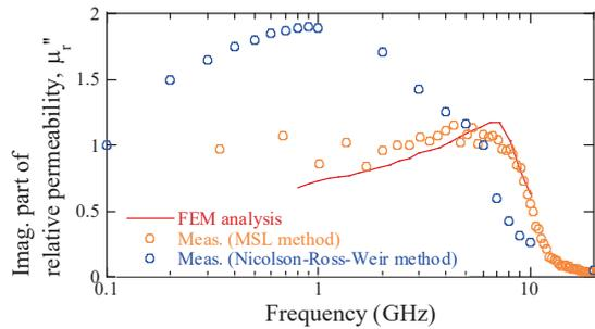
**Fig. 11** Simulated  $\mu_r''$  using FEM and measured data. The solid line is calculated using FEM and the square symbols show the data measured with the NRW method for comparison. The simulation predicted the shift of the FMR frequency. The measured spectrum using an MSL probe roughly agreed with the simulation data.
