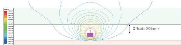
(a) magnetic flux line on 0.36 mm probe
