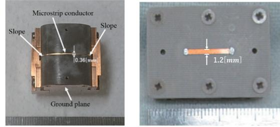
**Fig. 3** Photo of the MSL probe. This probe has a narrow microstrip line (0.36 mm wide (left)<sup>16)</sup> and 1.2 mm wide (right)<sup>22)</sup> and copper block as return pass.
