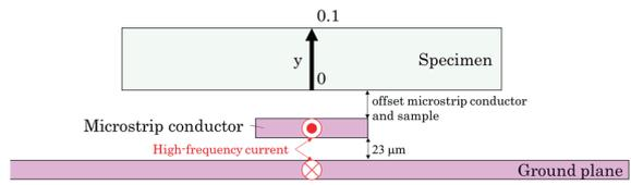
**Fig. 8** Calculation model and evaluation of the demagnetizing factor. “y” is the distance from the center point of the specimen on the side of strip line to the opposite surface, the thickness of which is assumed to be 0.1 mm.
