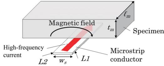
**Fig. 1** Configuration of MSL probe.
