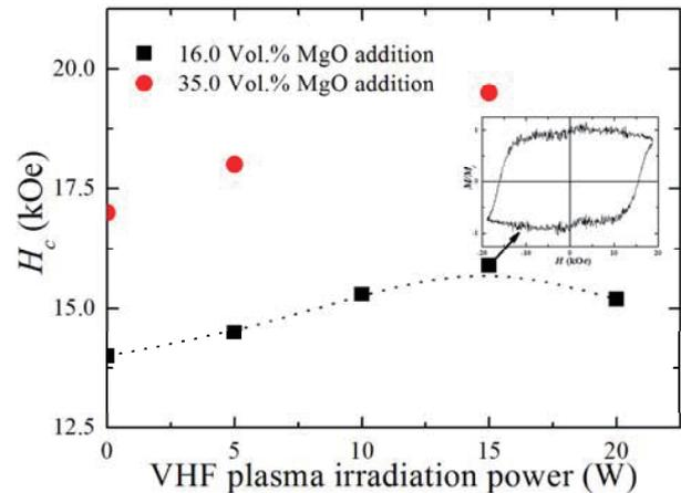
**Fig. 5** Dependence of the in-plane coercivity of FePt•MgO films on the VHF plasma irradiation power. The inset is hysteresis loop of (FePt)<sub>84</sub>•(MgO)<sub>16</sub> with VHF plasma irradiation power of 15 W.
