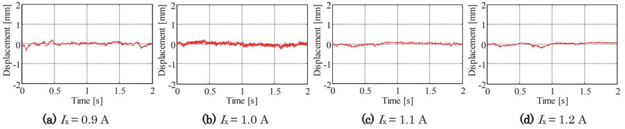
**Fig. 11** Time histories of the horizontal displacement  $x$  of the steel plate.
