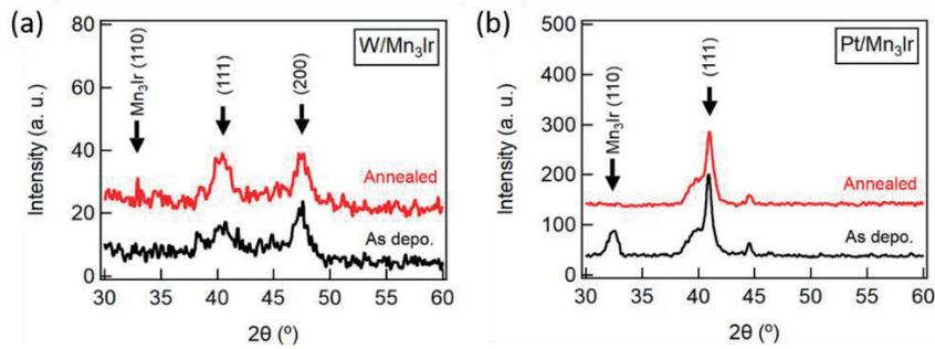
**Fig. 1** XRD patterns for (a)W 6 nm/Mn<sub>3</sub>Ir 30 nm/MgO 2 nm/W 2 nm and (b)Pt 6 nm/Mn<sub>3</sub>Ir 30 nm/MgO 2 nm/W 2 nm. The black line shows the result of the as deposited film and the red line is the result of the annealed film.
