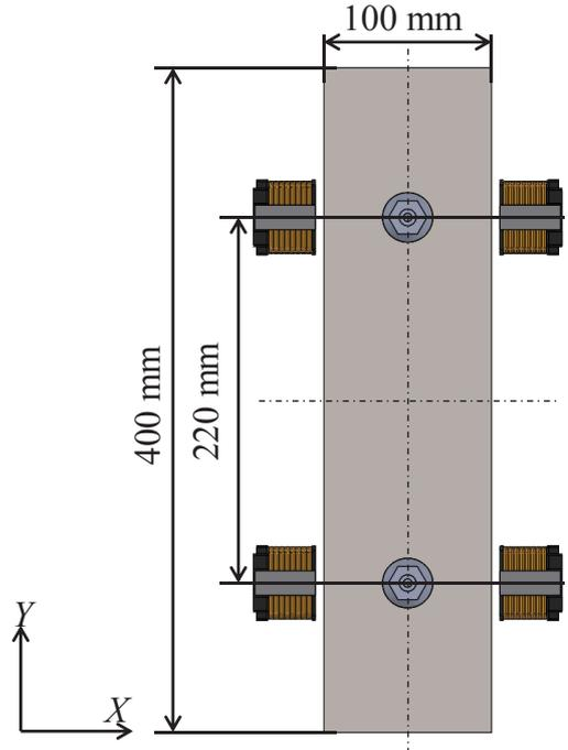
**Fig. 4** Placement of electromagnet and displacement field sensor.
