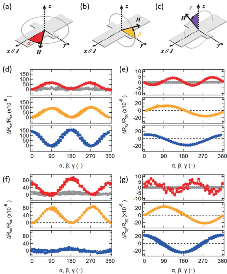
**Fig. 2** (a-c) Experimental setup of the electrical transport property measurement and the definition of the coordinate system.  $H$  denotes the magnetic field. (d,e) Angular dependence of  $R_{xx}$  and  $R_{xy}$  under the 9 T field at  $T=300$  K for the as-deposited (gray data points) and annealed W 6 nm/Mn<sub>3</sub>Ir 10 nm/MgO 2 nm/W 6 nm (f,g) and for the as-deposited (gray dots) and annealed Pt 6 nm/Mn<sub>3</sub>Ir 10 nm/MgO 2 nm/W 6 nm.
