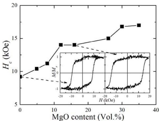
**Fig. 4** The in-plane coercivity versus MgO volume fraction in FePt•MgO films. The inset shows hysteresis loops of FePt and (FePt)<sub>84</sub>•(MgO)<sub>16</sub> film.
