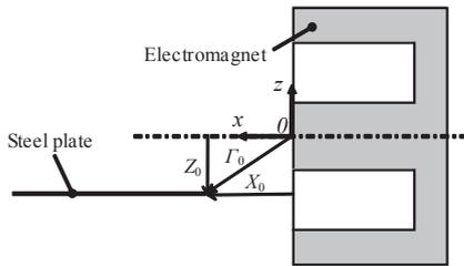
**Fig. 8** Coordinate of static levitating steel plate.
