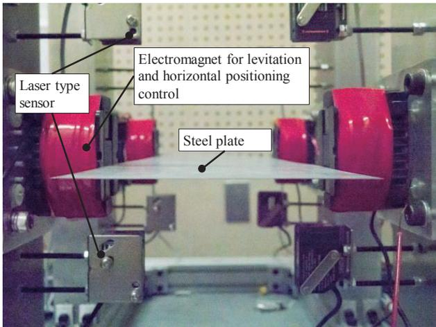
**Fig. 3** Photograph of the electromagnetic levitation system.
