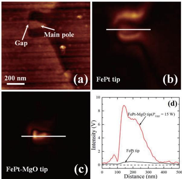
**Fig. 6** (a) is a topographic image, (b) and (c) are amplitude images of the AC magnetic field for the magnetic write head, and (d) is down track line profiles of amplitude signal of the white line in (b) and (c). The images in (b) and (c) are obtained using the FePt- and FePt·MgO-coated tips, respectively.
