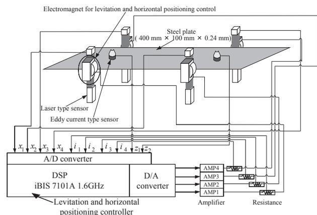
**Fig. 1** Edge supported levitation system for steel plate using only electromagnets installed horizontally.
