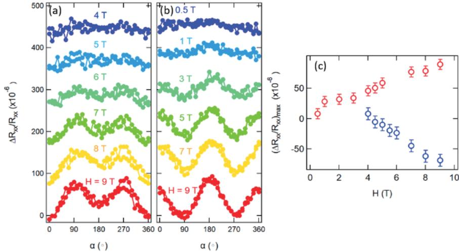
**Fig. 3** Field dependence of the magnetoresistive signals in the annealed W/Mn<sub>3</sub>Ir(a) and Pt/Mn<sub>3</sub>Ir(b) samples. (c) These magnetoresistance ratios are summarized as a function of magnetic field in red dots (Pt/Mn<sub>3</sub>Ir) and blue dots (W/Mn<sub>3</sub>Ir).
