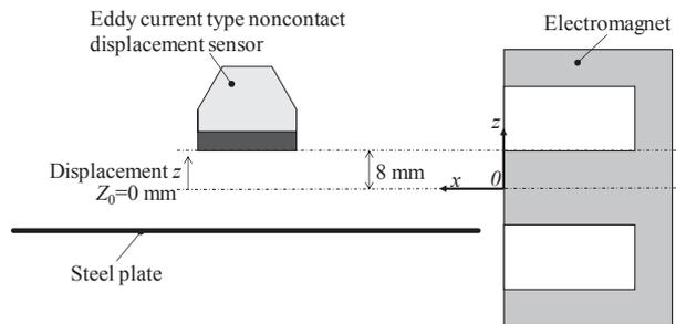
**Fig. 6** Position of eddy current type noncontact displacement sensor.
