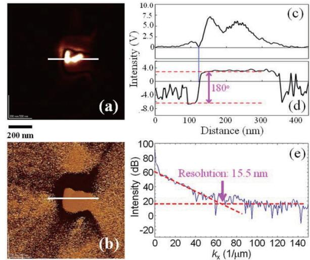
**Fig. 7** (a) amplitude and (b) phase images of the AC magnetic field for the magnetic write head measured by 20 nm  $(\text{FePt})_{84} \cdot (\text{MgO})_{16}$ -coated tip. (c) and (d) are down track line profiles of amplitude and phase signal of the white line in (a) and (b), respectively. (e) is the spatial resolution result of the amplitude image.
