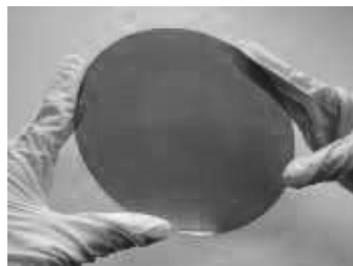
Fig.2 φ6 inch-sized Bi-substituted iron garnet film for MO imaging.
