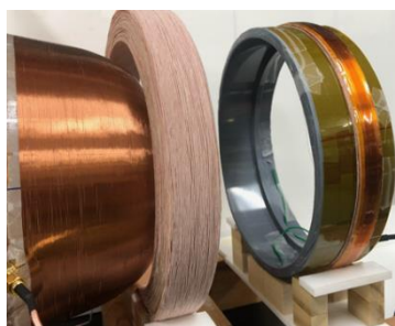
Fig. 1 Coil system for head-size magnetic particle imaging.
