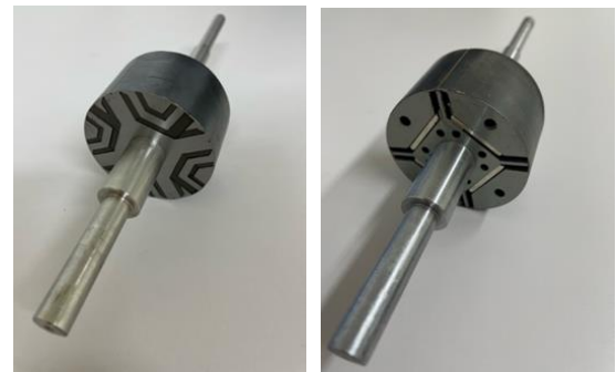
(a)Asymmetric IPM (b)Conventional IPM Fig.1 Appearance of the rotors.
