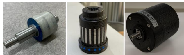
(a) Inner rotor (b) Pole-pieces (c) Magnetic gear
