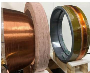
Fig. 1 Coil system for head-size magnetic particle imaging.
