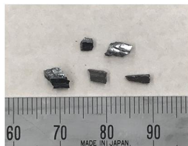
Fig. 1 \text{SrCo}_2\text{W} crystals obtained by FZ method in high oxygen pressure
