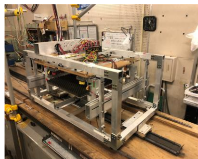
Fig. 1 Photograph of conveyance system of the steel plate
