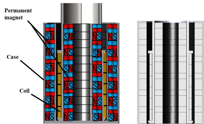
(a) Schematic of the actuator (b) Shape of the array at 2:1
