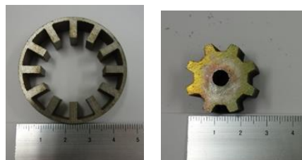
Fig. 2. Stator and rotor cores of SMC-based SR motor manufactured by using wire electric discharge machining.
