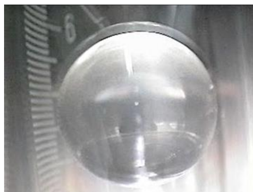
Figure 2. Levitation of water by magneto-Archimedes levitation
