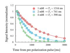
Fig. 2 Measured relaxation curves and calculated relaxation time of  $NiCl_2$  aqueous solution phantoms.
