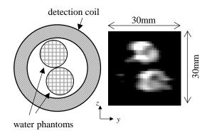
Fig. 1 Magnetic resonance image of water phantoms taken by the detection coil at 70  $\mu$ T.
