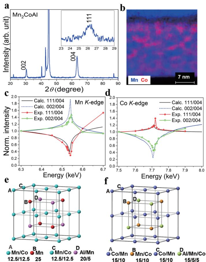
Fig.1 (a) Lab. XRD patterns of  $\text{Mn}_2\text{CoAl}$  films fabricated by MBE. Inset: 111 reflection profile. (b) STEM-EDS mapping of Mn and Co in  $\text{Mn}_2\text{CoAl}$  film. Calculated and experimental anomalous XRD  $I_{111}/I_{004}$  and  $I_{002}/I_{004}$  profiles at (c) Mn  $K$ -edge and (d) Co  $K$ -edge. Crystal structures of (e) Mn -rich phase ( $L2_1B$  structure) and (f) Co-rich phase (disordered  $L2_1$  structure).
