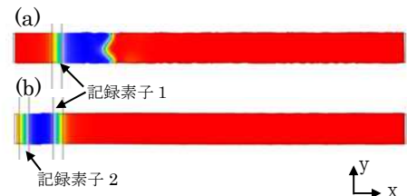
Fig.2 Simulation results of domain formation in specimen nanowires with (a) recording head 1, and (b) with recording heads 1 & 2 with a separation distance of 100 \text{ nm} , respectively.
