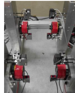
Fig. 1 Photograph of the electromagnetic levitation system.
