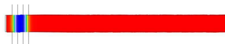
Fig.3 Simulation result of domain formation in specimen nanowire with recording heads 1 & 2 with a separation distance of 40 \text{ nm} .
