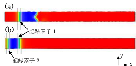
Fig. 2 Simulation results of domain formation in specimen nanowires with (a) recording head 1, and (b) with recording heads 1 & 2 with a separation distance of 100 \text{ nm} , respectively.
