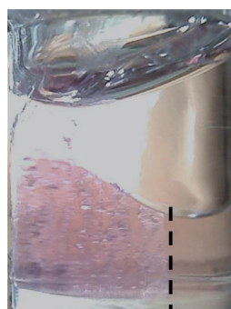
Fig. 4 Side view of the vertical interface under horizontal gradient magnetic field. the interface was indicated as broken line.
