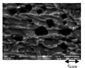
Fig. 2 Magneto-drill effect on a copper rod electrode at 10T.
