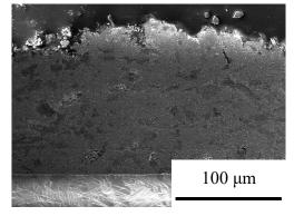
Fig. 2 Cross-sectional SEM image of Al<sub>2</sub>O<sub>3</sub>-Ni composite film formed by CCMFP; darker gray parts are included Al<sub>2</sub>O<sub>3</sub> particles.
