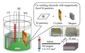
Fig. 1 Experimental setup of the three-electrode electrochemical cell for CCMFP with a Cu plate working electrode with magnetically fixed Ni particles, a Ni wire quasi reference and a Ni counter electrode. Photos of the magnet A and B, and the schematic structure of the magnet B are also presented.
