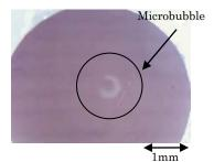
Fig 1. Microbubble globules on copper surface during copper dissolution at 8 T.
