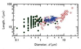
Fig. 2 Scatter plot for fullerene nano rod crystallized under the influence of magnetic fields. The symbols  $\bullet$ ,  $\times$ , and  $\circ$ , corresponded to the size for Fig. 1(a), (b) and (c), respectively.
