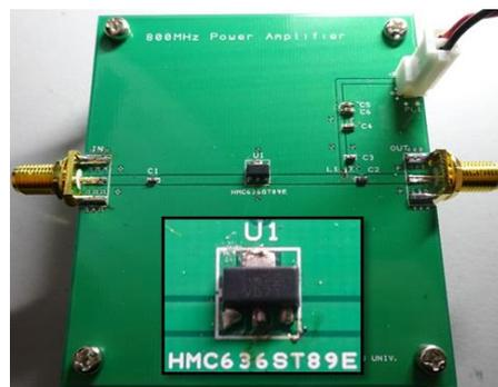
Fig. 2 DUT "RF power amplifier"
