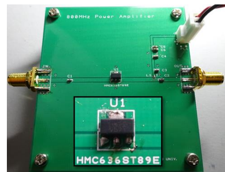
Fig. 2 DUT "RF power amplifier"
