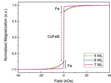
Fig. 1. Magnetizations as a function of in-plane magnetic fields for ultrathin-Fe/MgAl<sub>2</sub>O<sub>4</sub>/CoFeB MTJs with 5-7 ML thick Fe.
