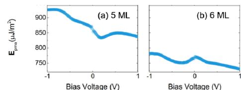
Fig. 2. Bias voltage dependences of  $E_{pma} = K_{eff} \times t_{Fe}$  for (a) 5-ML and (b) 6-ML Fe sample.
