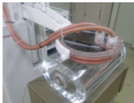
Fig. 1 Pancake-type applicator and human-body phantom.
