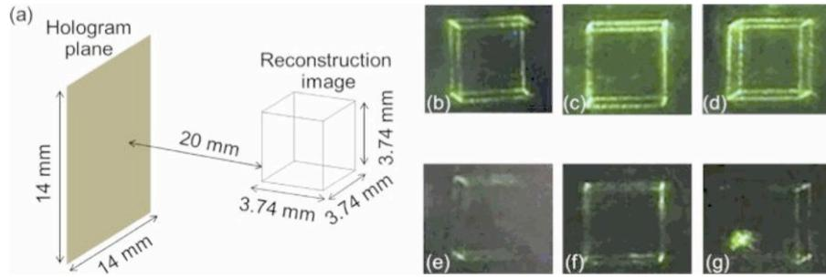
Fig. 1 (a) A model of 3D image for generating the hologram. The wireframe cube was constructed by point light sources. (b)–(d) Reconstructed images from MPC and (e)–(g) those from *a*-TbFe for comparison. The images of (b) and (e) were from left view point of  $11^\circ$ , (c) and (f) were from center, and (d) and (g) were from right view point of  $11^\circ$ .
