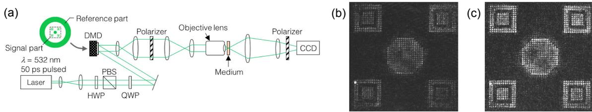
Fig. 2. Experimental setup and reconstructed two-dimensional data patterns. (a) Schematic illustration of the experimental setup for writing and reconstructing magnetic holograms. Reconstructed signal patterns from (b) the single layer Bi:RIG film and (c) the two-pair MPC medium. The MPC medium provided a clear and bright image because the diffraction efficiency of MPC medium was as double as that of the single layer film.
