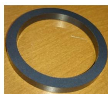
Fig. 3 Specifications of a ring core of SMC.
