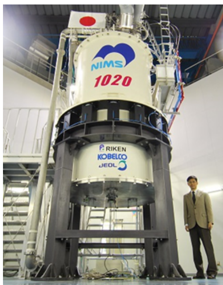
Fig.1 1020 MHz-NMR magnet. It weighs 15 tons, 5 meters in height and has a high temperature superconducting coil inside.
