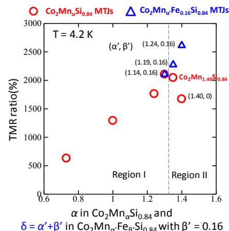
Fig. 2. TMR ratios of CMFS-based MTJs as a function of  $\delta = \alpha' + \beta'$  in  $\text{Co}_2\text{Mn}_{\alpha'}\text{Fe}_{\beta'}\text{Si}_{0.84}$  electrodes and that of identically fabricated CMS-based MTJs as a function of  $\alpha$  in  $\text{Co}_2\text{Mn}_{\alpha}\text{Si}_{0.84}$  electrodes.
