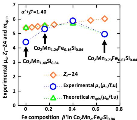
Fig. 1. Saturation magnetization per formula unit of  $\text{Co}_2\text{Mn}_{1.40}\text{Si}_{0.84}$  and  $\text{Co}_2\text{Mn}_{\alpha'}\text{Fe}_{\beta'}\text{Si}_{0.84}$  films with  $\alpha' + \beta' = 1.40$  in comparison with Slater-Pauling value ( $Z_{\uparrow-24}$ ) and theoretical  $m_{\text{spin}}$ .
