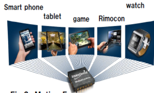
Fig.2 Motion Fusion sensor size 4×4×1mm
