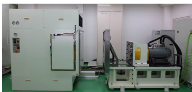
Fig. 2 High-precision motor-loss evaluation system.
