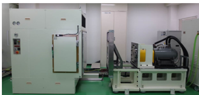
Fig. 2 High-precision motor-loss evaluation system.
