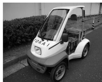
Fig. 1 Ultra-compact electric vehicle
