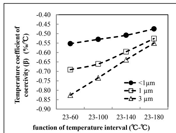
Fig.1 Variation of  $\beta$  of the Nd-Fe-B sintered magnet vs a function of temperature interval.
