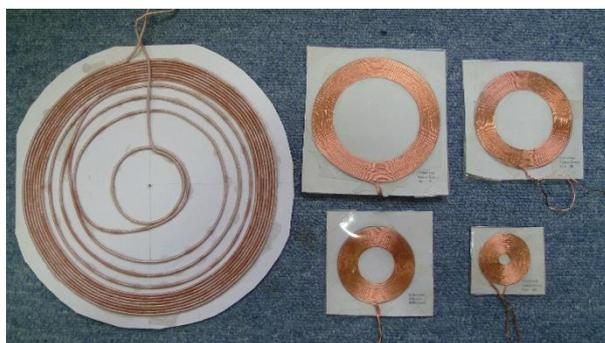
Fig. 1. Proposed station coil in supply side.
