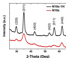
Fig. 1: XRD patterns of N10x and N10x-1H
