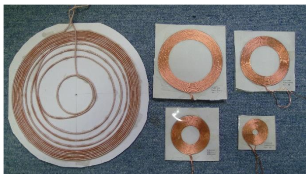
Fig. 1. Proposed station coil in supply side.
