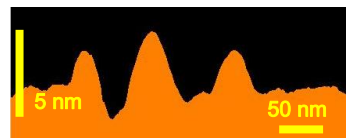
Fig.4 AFM cross section profile of silica particle on FePt continuous film ( t_e = 10 s).
