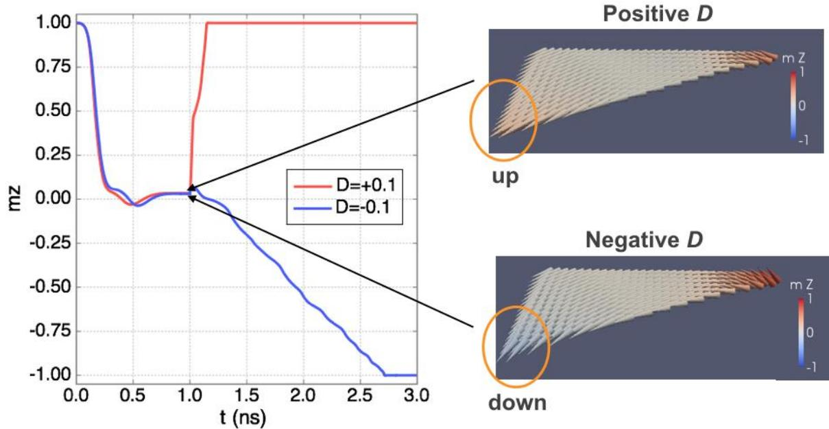
Fig. 2 Temporal variation of the z-component of the averaged magnetization,  $m_z$ , and snap shots of magnetization at the end of the pulse duration. The result for positive (negative) bias voltage is represented by the solid red (dotted blue) curves.
