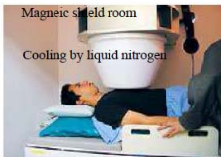
Fig.3 magnetocardiography using SQUID
