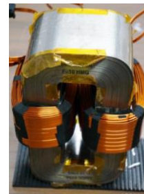
Fig. 3 Appearance of the test amorphous transformer.
