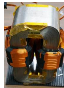
Fig. 3 Appearance of the test amorphous transformer.
