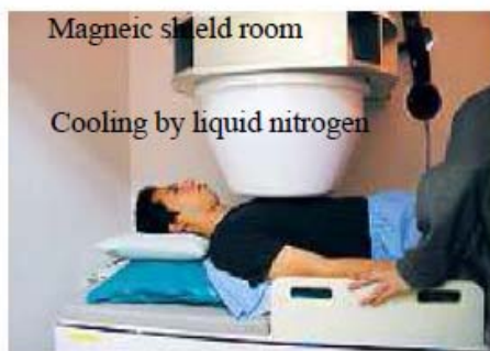
Fig.3 magnetocardiography using SQUID
